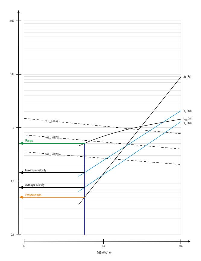
Q – Air outlet for a single 1m long diffuser.
